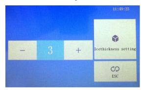
Press SETUP-> USER SETUP - > ICE THICKNESS ADJUST icon to enter the ice thickness setting interface; press + or - to increase or decrease the ice thickness(+or-represents the
