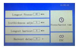
■ Longest Freeze: This parameter specifies the maximum ice making time. When the ice making time is greater than this value, the ice maker forces de icing. If the time-out is 3 times in succession, the ice maker will stop working and give a fault alarm
